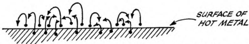
Fig. 1: Electrons being emitted from the surface of hot metal
